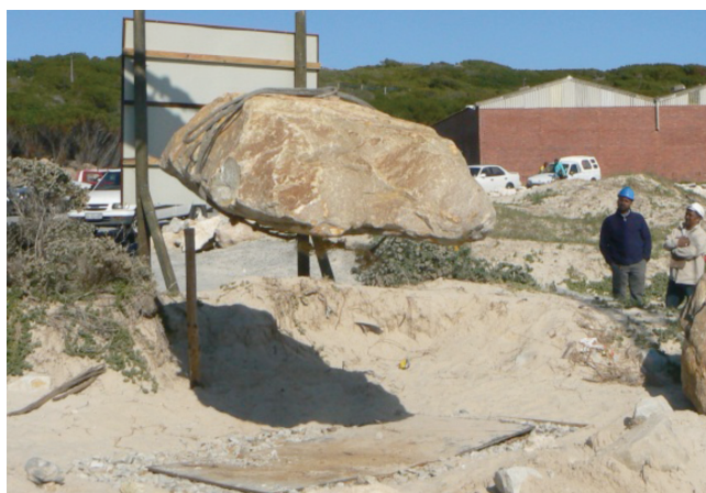
1.5 m high drop test. Steel plate on crushed rock.
