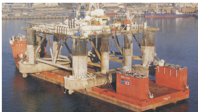
Ship repairer ingenuity: semi-sub on a heavy lift vessel.
